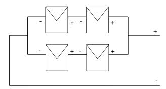
Note: When a project is wired with modules in parallel, it is important to check the fuse rating of the module. This value is available on the module's label as well as on the dedicated data sheet. Indeed, in case of 1 line shadowing, the line that is still producing energy will "load" the other. This is why an appropriate line fuse protection must be applied and follow appropriate standards.
