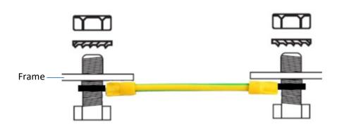
It is recommended to use a 10 mm<sup>2</sup> bonding connector to realize the grounding between each module. The recommended section to the main equipotential bonding is 16 mm<sup>2</sup>.
