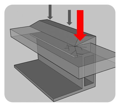
When clamping, please make sure that force is homogenously shared on aluminium part. Force cannot deform top frame flange. For module series equipped with a water drain corner, clamp must not be applied directly on.
