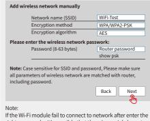
If the Wi-Fi module fail to connect to network after enter the right passwords. It's possible that there is special characters not supported by module in the hotspot passwords.
