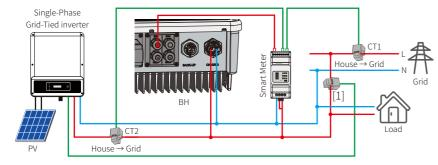
[1] This cable is a theoretical connection supporting anti-reverse function, which could be different for different grid-tied inverters.
