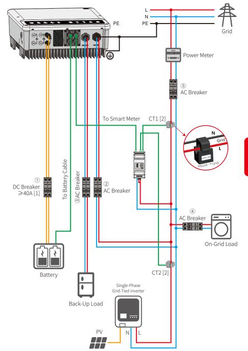
Note: According to australian safety country, the neutral cable of on-grid side and back-up side must be connected together, otherwise back-up function will not work.
