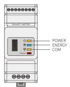
The Smart Meter with CT in product box is compulsory for BH system installation, used to detect grid voltage and current direction and magnitude, further to instruct the operation condition of BH inverter via RS485 communication.
