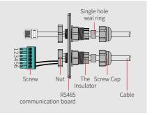
Connect the terminal to the right position onto the inverter.
