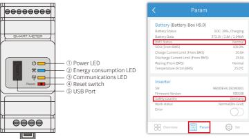
Note: For compatible lithium batteries, BMS status will display "Normal" after selecting the right battery company.
