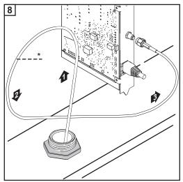
\*Bending radius of the antenna cable: at least 25.4 mm/1 in.
