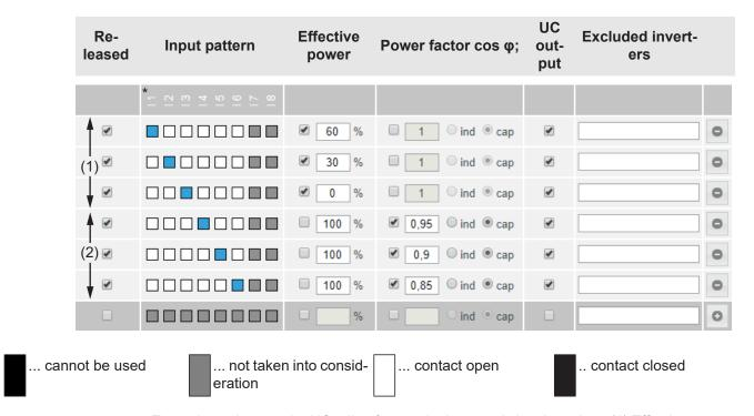
Example settings on the UC editor for two ripple control signal receiver: (1) Effective power limitation,
