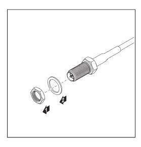
Remove the hex nut and washer from the outside thread of the antenna cable
