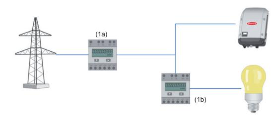
A meter for recording self-consumption per S0 can be connected directly to the inverter.
