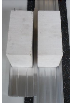
Figure 43 Ballast distribution on base troughs (left) or via ballast trough (right)
