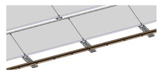
To reduce ballast on the southern (East-West) edge or at interruptions in the system (e.g. along light domes or maintenance walkways), place a base trough 150-30 rectangular on the base troughs as a connection rail and each with two screws per base trough. Extension using base trough connectors or expansion joints at system interruptions. Arrange the expansion joints identically to the expansion joints of the module supports. Cut the base troughs to length if required.
